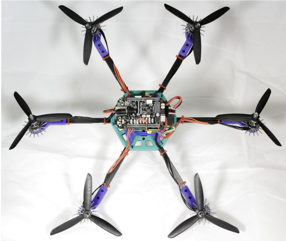
Figure 5.5: Top view of case study airframe with optimized angles as used for experiment.
