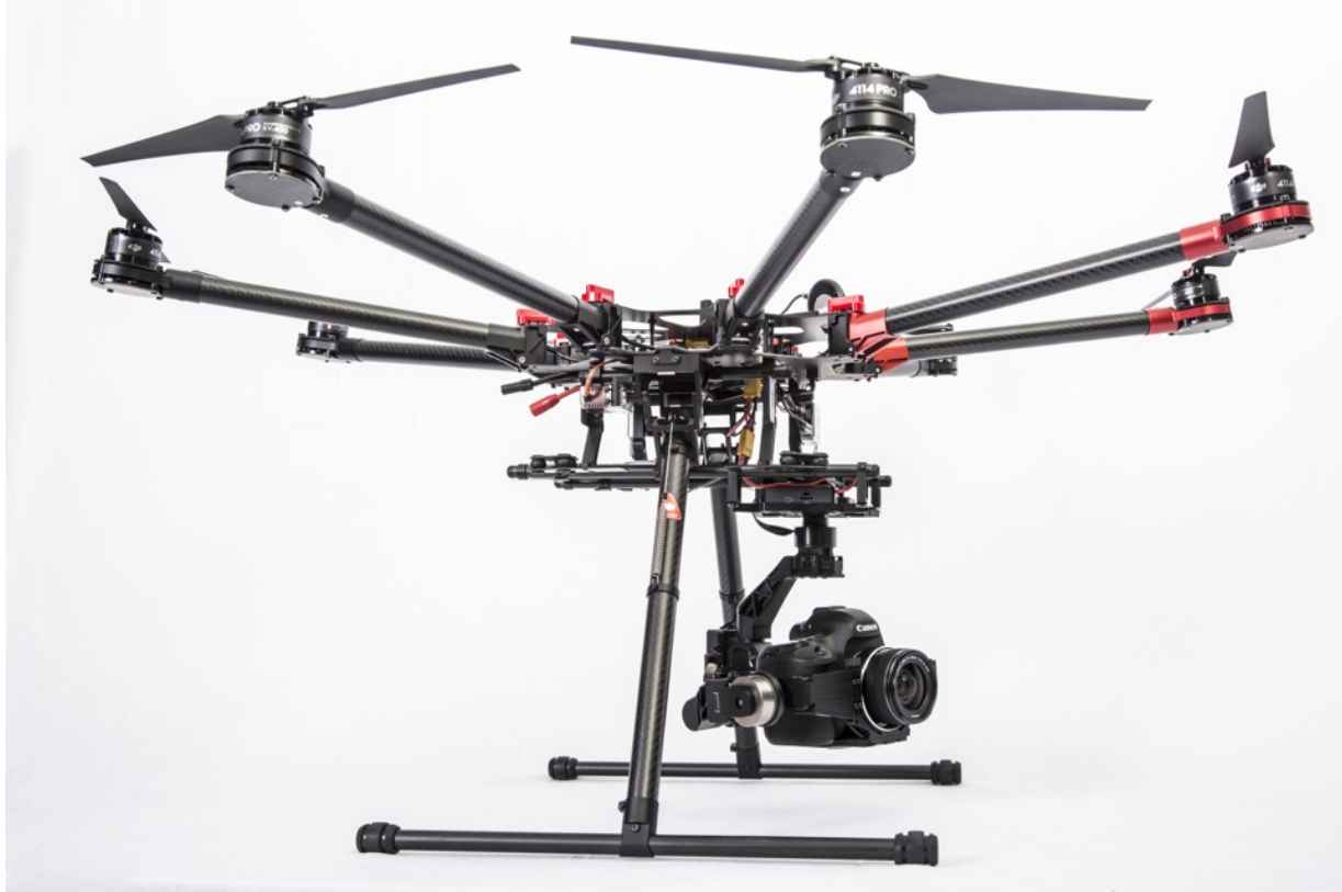
Figure 3.4: DJI S1000 multirotor frame demonstrating low center of mass and inward tilt of rotors.
